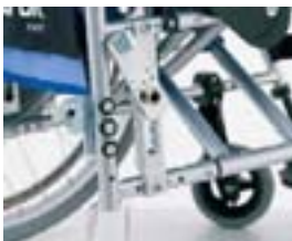
The power hubs fit the chair similar to ordinary wheels
